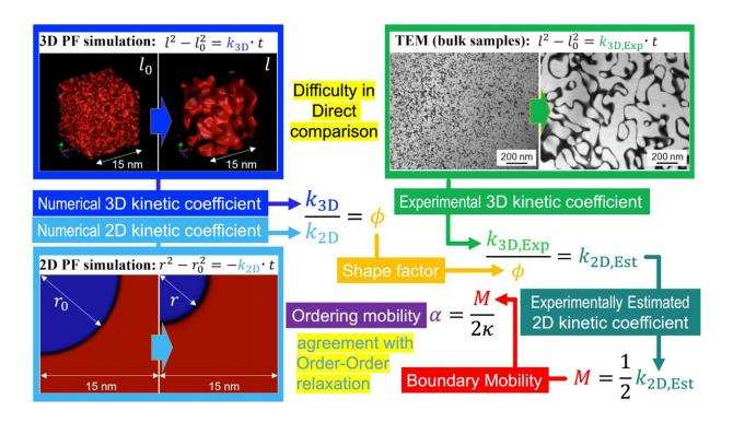
Comparison of simulations and experiments for AntiPhase Boundary (APB) migration and derivation of the shape coefficients. Credit: 2024 Koizumi et al., Resolving the long-standing discrepancy in Fe<sub>3</sub>Al ordering mobilities: A synergistic experimental and phase-field study. *Acta Materialia*
