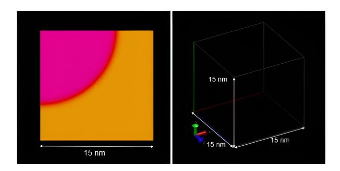
PF simulations imitating the process of circular APB shrinking in 2D space (left) and APD growth in 3D space (right). Credit: 2018–2024 Koizumi Lab. Osaka University, All rights reserved.
