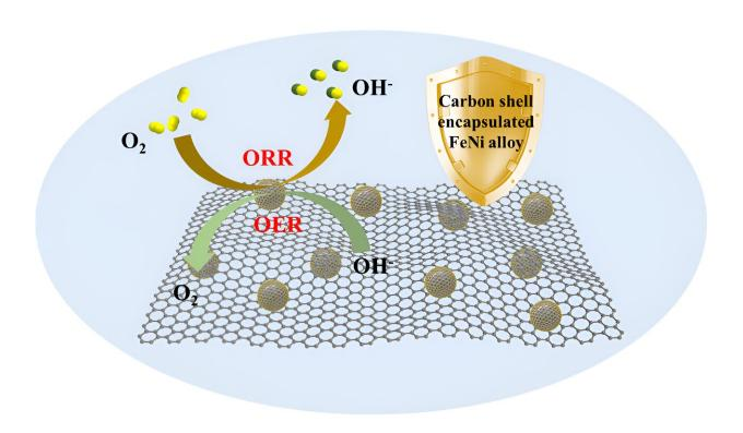
FeNi alloy nanoparticles, encapsulated in a carbon shell and supported on N-doped graphene nanosheets, have been prepared. This chainmail catalyst demonstrates superior performance in oxygen reduction and evolution reactions, and Zn-air batteries. This enhanced performance is attributed to the synergistic effect between the shell and the alloy. Credit: Chinese Journal of Catalysis
