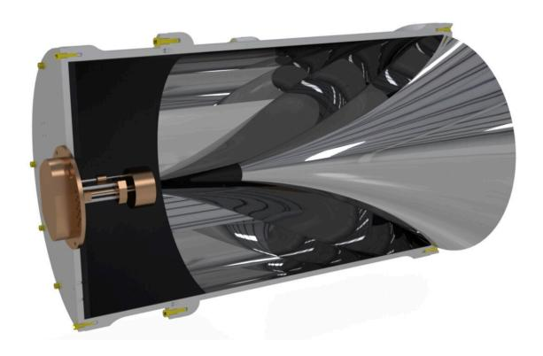
A rendering of the BREAD design. The "Hersheys Kiss"—shaped structure funnels potential dark matter signals to the copper-colored detector on the left. The detector is compact enough to fit on a tabletop. Credit: BREAD Collaboration
