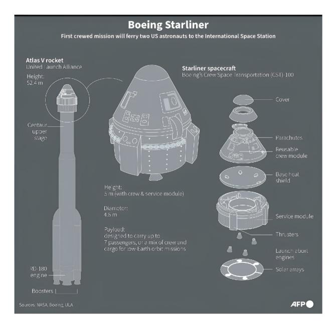
Graphic on the Boeing Starliner, which will make its first crewed mission to the International Space Station on the Atlas V rocket.
