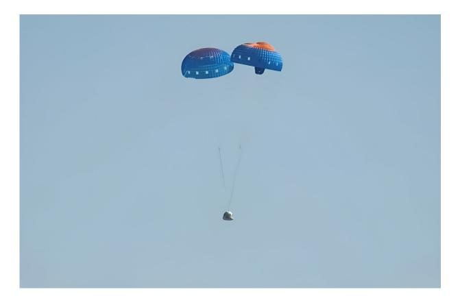
One of the Blue Origin capsule's three parachutes failed to fully inflate, possibly resulting in a harder landing than expected.
