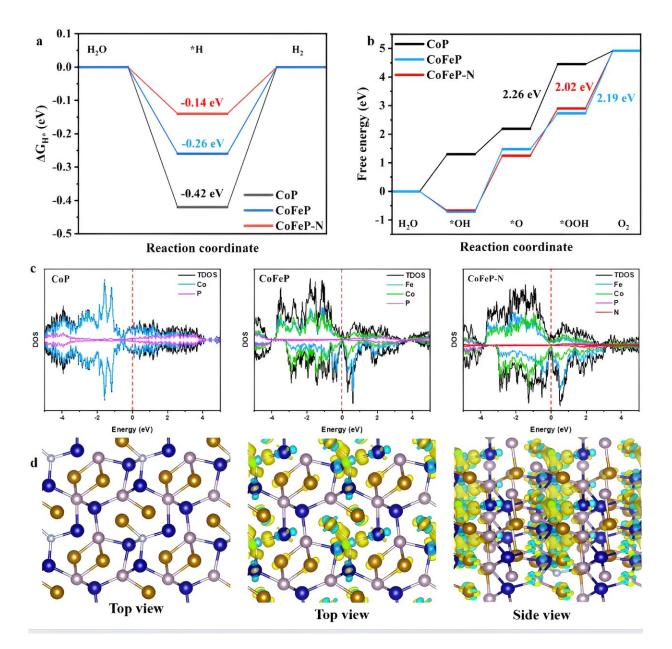
Theoretical calculations illustrate the efficient electrocatalytic water splitting mechanism of CoFeP-N nanowires. Credit: Wang Ruiqi
