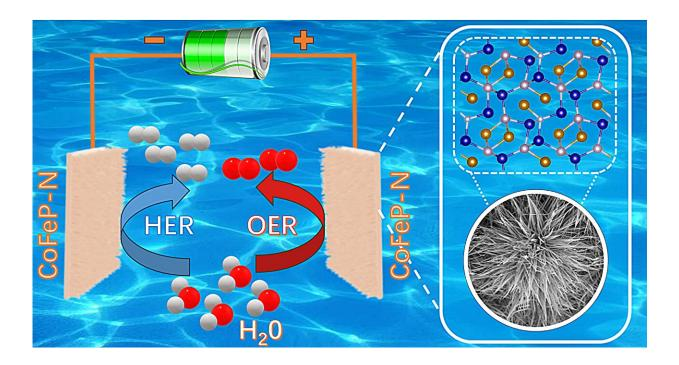
Schematic diagram of efficient electrocatalytic water splitting by CoFeP-N nanowires. Credit: Wang Ruiqi
