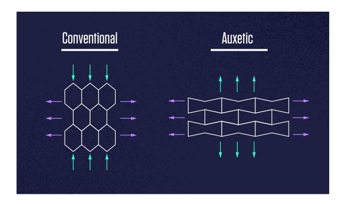
Auxetics defy common sense. Unlike conventional materials, which narrow when pulled lengthwise, they widen when pulled lengthwise. Credit: N. Hanacek/NIST
