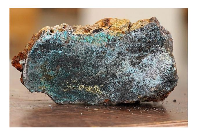
Take a close look at these seabed minerals! Green copper minerals are seen here precipitated in a sectioned sulphide sample, retrieved from a scientific cruise conducted by the Norwegian Offshore Directorate across the Mohns Ridge in 2020. Credit: Øystein Leiknes Nag/Norwegian Offshore Directorate
