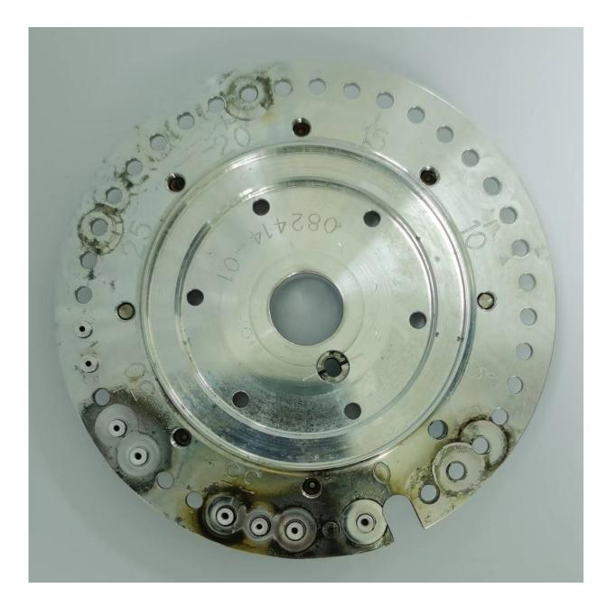
The cathode holder disk is part of the NEC multi-cathode source of negative ions by cesium sputtering. Cathodes of <sup>60</sup>Fe samples and blank samples were installed on the holder disk. Credit: China Institute of Atomic Energy
