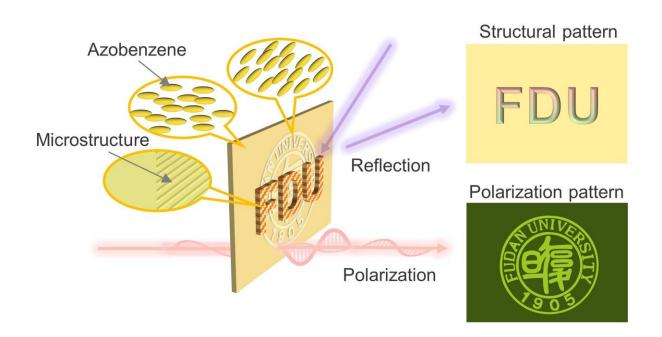
A new dual-mode security film reveals one image when light reflects off a pattern stamped on its surface, and a second image when polarized light shines through it. Credit: Adapted from Langmuir 2024, DOI: 10.1021/acs.langmuir.4c01297
