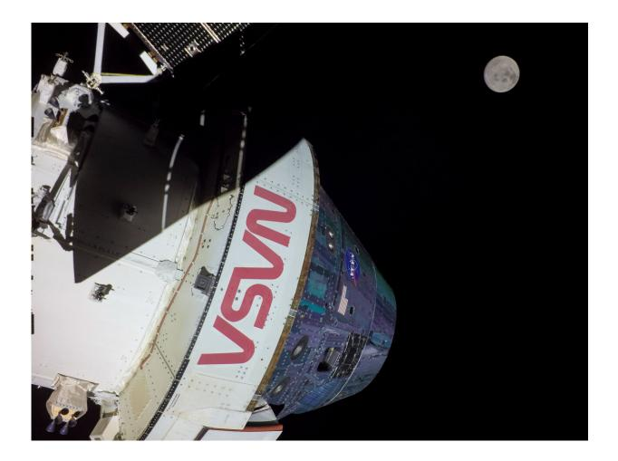
On the 19th day of the Artemis I mission, the moon grows larger in frame as Orion prepares for the return powered flyby on Dec. 5, when it will pass approximately 79 miles above the lunar surface. This image includes both the Orion crew module and service module, connected by the compression pad that utilizes the 3D-MAT material. Credit: NASA
