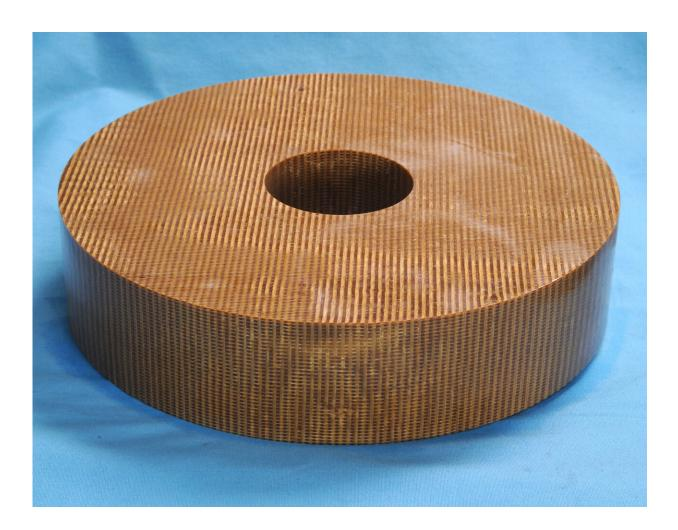
The 3D-MAT thermal protection material. Credit: NASA
