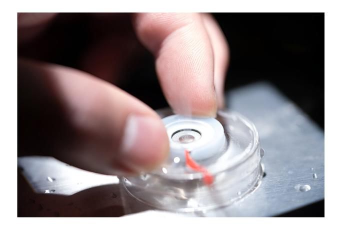
Researchers at MIT have discovered a new phenomenon: that light can cause evaporation of water from its surface without the need for heat. Pictured is a lab device designed to measure the "photomolecular effect," using laser beams. Credit: Bryce Vickmark
