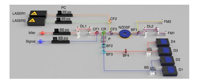
Experimental setup of the NOON-state interference. PC polarization controller, DL delay line, CF combining filter, CR circulator, NZDSF non-zero dispersionshifted fiber, BF bandpass filter, FM Faraday mirror, P polarizer, BS beam splitter, D superconducting nanowire single-photon detector. Credit: *Light: Science & Applications* (2024). DOI: 10.1038/s41377-024-01439-9
