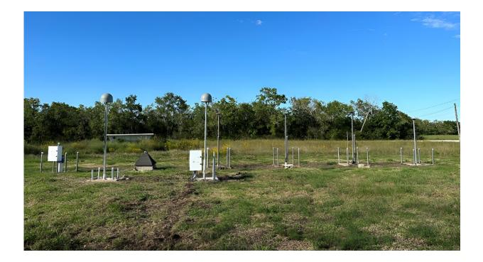
GPS array at the University of Houston Coastal Center, which has been continuously operated for 10 years, providing first-hand observations for the study. Credit: University of Houston
