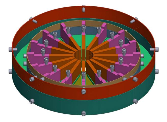
The design of the mechanical assembly of the magnetic optics section for APES-360. The actual magnets are the orange rectangles near the middle. The entrance aperture is a gap between the green and red outer bands. Credit: NASA GSFC
