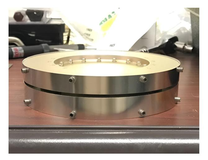
Magnet assembly of prototype APES-360 instrument for simultaneously measuring electron spectra in 16 different directions. Credit: NASA GSFC
