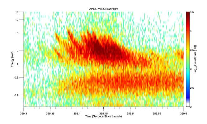
Precipitating electron spectra measured inside the aurora at one millisecond time resolution using the APES instrument on the Visualizing Ion Outflow via Neutral Atom Sensing-2 (VISIONS-2) sounding rocket flight. This entire plot covers a period of 300 milliseconds. The slanted red stripes in the middle of the figure are on the order of 10 milliseconds apart. Credit: NASA GSFC
