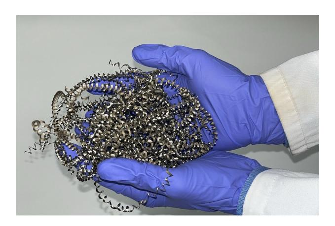
Waste metal swarf used in experiment to transform it into a highly efficient catalyst to make hydrogen from water, a discovery that could make hydrogen production more sustainable. Credit: University of Nottingham
