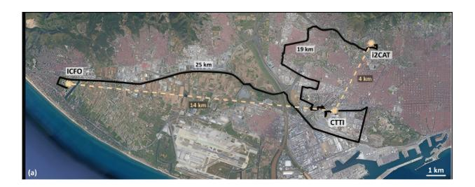
Measurement of non-classical correlations between remote locations. Map of the metropolitan area of Barcelona, with the three locations highlighted: ICFO, where the memory and SPDC source are located; CTTI, where the two optical fiber segments are connected; i2CAT, where the idler photons are detected. Credit: ICFO
