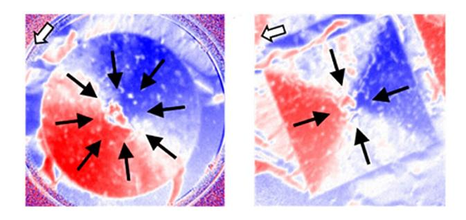
The radially aligned spin textures in a round and a square sample consisting of a ferromagnetic material on a superconducting YBCO island. The white arrow shows the incident X-ray beam. Credit: HZB
