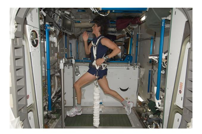
NASA astronaut Sunita Williams, Expedition 32 flight engineer, equipped with a bungee harness, exercises on the Combined Operational Load Bearing External Resistance Treadmill (COLBERT) in the Tranquility node of the International Space Station. Credit: NASA
