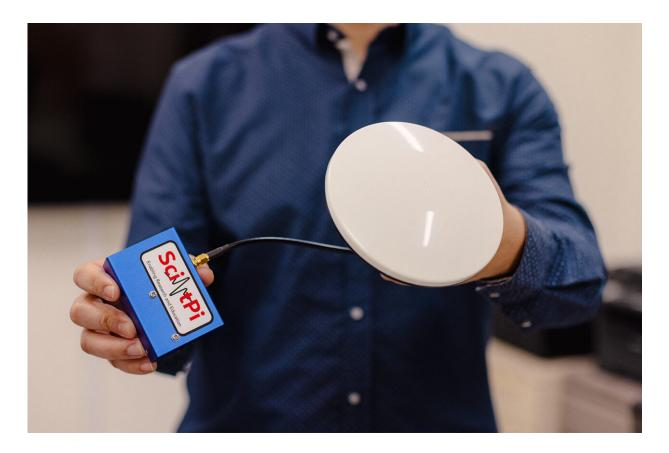
Josemaría Gómez Sócola displays a ScintPi sensor and its antenna. The sensors have been deployed at 23 sites across the Western Hemisphere so that scientists can study the ionosphere at low, medium and high latitudes. Credit: University of Texas at Dallas
