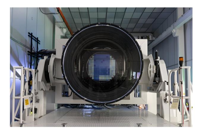
A front view of the completed LSST Camera, showing the 3,200-megapixel focal plane within. Credit: Jacqueline Ramseyer Orrell/SLAC National Accelerator Laboratory
