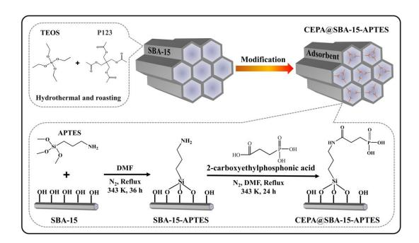
Schematic illustration of CEPA@SBA-15-APTES preparation process. Credit: Zhang Shichang
