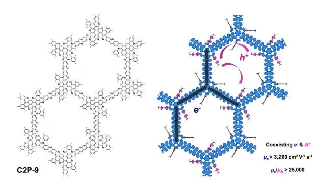
Diagram depicting the chemical structure of a conducting two-dimensional polymer (C2P-9) with pendant groups and the coexistence of ultrafast electrons after p-type doping. Credit: POSTECH
