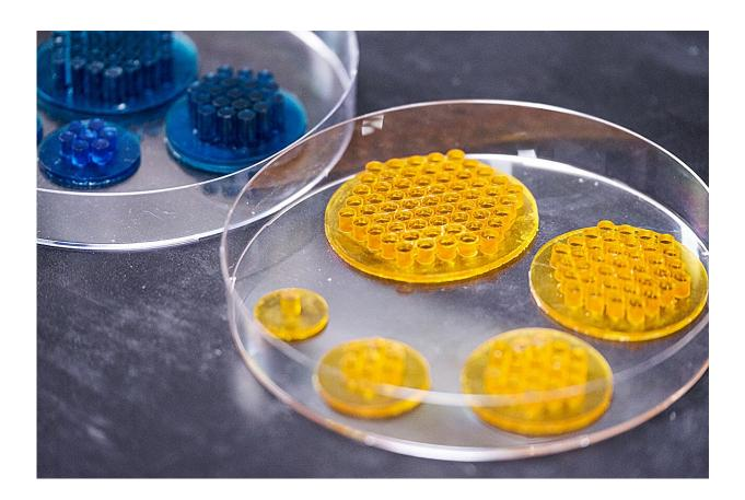
The NTU team designed shape-memory polymers, which are smart materials that can 'remember' their previous forms, in the form of hair-like fibrils which they found in their testing to provide maximum adhesive strength. Credit: Nanyang Technological University
