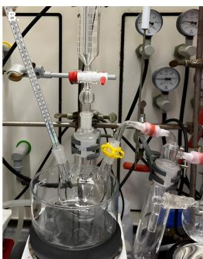
A) Reaction set-up for the preparation of NO<sub>2</sub>Cl. B) A 250-mL three-necked round-bottomed flask was equipped with a thermometer, a 50-mL dropping funnel, a stir bar, and connected to a 200mL Schlenk flask equipped with a bubbler. Credit: *Science* (2024). DOI: 10.1126/science.adn7006
