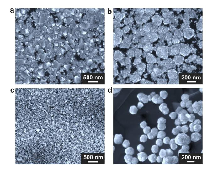
Diamonds of various morphologies as grown under different growth conditions. (a) Growth by using a liquid metal alloy of Ga/Ni/Fe/Si (77.75/11.00/11.00/0.25 at%) under methane/hydrogen (1/20 molar ratio). (b) Growth by using a liquid
