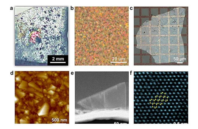
Growth of diamond in liquid metal alloy under 1 atmosphere pressure. (a) A photo showing the as-grown diamond on the solidified liquid metal surface. (b) An optical image of the as-grown continuous diamond film on the solidified liquid metal surface. (c) An optical image of the as-transferred diamond film on a Quantifoil holey amorphous carbon film coated Cu TEM grid. (d) An atomic force microscopy topographic image of the as-transferred diamond film on the
