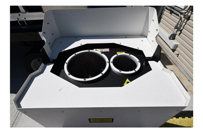
A top-down view of the lidar. A laser fires from the aperture on the right and then the telescope aperture on the left opens its "eye" briefly to collect photons backscattered from the atmosphere. Credit: Kevin Coughlin/Brookhaven
