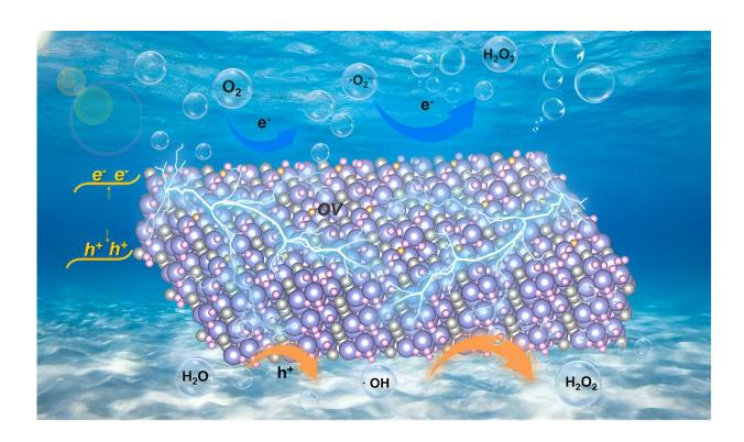
$Bi_4O_5Br_2$  is highly attractive as an efficient piezocatalyst that utilizes the ubiquitous mechanical energy for  $H_2O_2$  synthesis. Oxygen vacancies mediated ultrathin  $Bi_4O_5Br_2$  nanosheets display a better piezoelectric response and stronger adsorption and activation ability of oxygen, leading to an outstanding piezocatalytic  $H_2O_2$  synthesis performance without any sacrificial agents and cocatalysts in pure water. Credit: Chinese Journal of Catalysis
