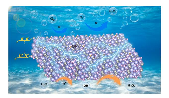
$Bi_4O_5Br_2$  is highly attractive as an efficient piezocatalyst that utilizes the ubiquitous mechanical energy for  $H_2O_2$  synthesis. Oxygen vacancies mediated ultrathin  $Bi_4O_5Br_2$  nanosheets display a better piezoelectric response and stronger adsorption and activation ability of oxygen, leading to an outstanding piezocatalytic  $H_2O_2$  synthesis performance without any sacrificial agents and co-catalysts in pure water. Credit: Chinese Journal of Catalysis
