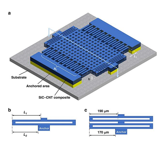
A schematic of the accelerometer. a Typical structure of a MEMS comb-type accelerometer, b single-meandered spring, c double-meandered spring. Credit: *Microsystems & Nanoengineering* (2024). DOI: 10.1038/s41378-024-00672-x
