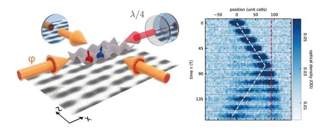
Using laser beams (yellow and red) the researchers create a lattice, in which the atoms are trapped (left) and transported through the lattice by topological pumping (right). Credit: Quantum Optics Group / ETH Zurich
