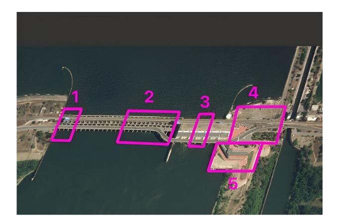
Using post-collapse images acquired by Umbra and pre- and post-collapse Sentinel-1 images, the University of Houston team identified two main breaches at the dam. Numbered portions depict the collapsed parts of the dam. Credit: University of Houston
