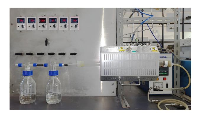
The flow-type fixed-bed reactor used in the process of recovering phosphorus from incinerated sewage sludge. Credit: Naoto Tsubouchi / Hokkaido University
