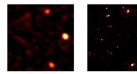
Old versus new. Left shows an image of a piece of sky observed with the hitherto best calibration technique. Right shows the same piece of sky with the new technique. More detail is visible, and what were once large, blurry patches now appear as single points. Credit: LOFAR/Groeneveld et al.
