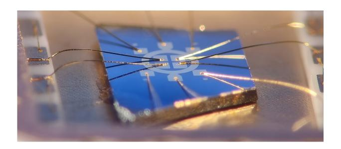
Until now, the zero magnetic field quantum anomalous Hall effect only occurred at very low currents. This device can change that. Credit: Kajetan Fijalkowski /JMU
