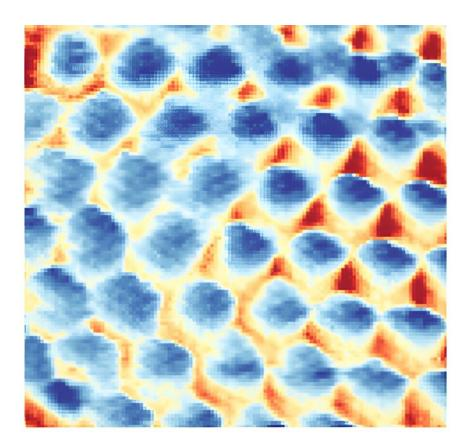
An image of a triangular Wigner crystal taken by scanning tunneling microscope. Researchers have unveiled an elusive crystal that is formed purely from the repulsive nature of electrons. Each site (blue circular region) contains a single localized electron. Image by Yen-Chen Tsui and team, Princeton University. Credit: Yen-Chen Tsui, Princeton University
