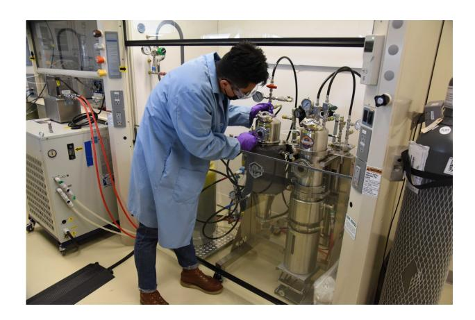
Loading the contaminated cardboard into the DME extraction chambers. Credit: Idaho National Laboratory
