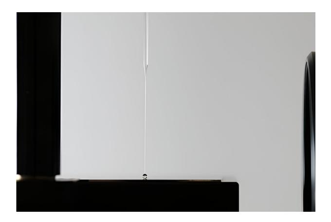
Assistant Physics Professor Matilda Backholm's unique micropipette force sensor technology probes the tiny forces acting between a superhydrophobic material and a water droplet. Credit: Matilda Backholm/Aalto University
