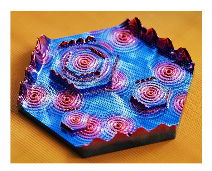
A representation of data visualization of quantum states of electrons on the surface and edge of gray arsenic crystal obtained using a scanning tunneling microscope at Princeton's physics department. Credit: Image based on STM data simulations prepared by Shafayat Hossain and the Zahid Hasan group at the Laboratory for Topological Quantum Matter at Princeton University.
