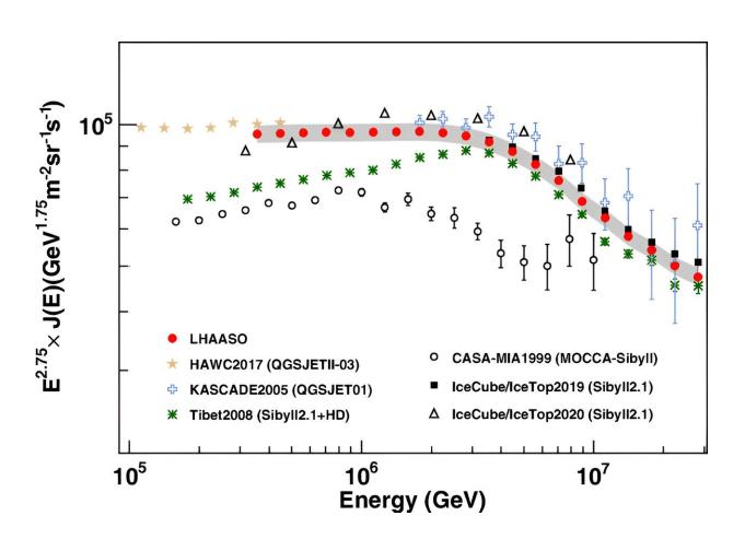
The LHAASO-KM2A all-particle energy spectrum flux multiplied by E<sup>2.75</sup> as a function of energy. The gray shadow band represents the estimated systematic uncertainties. The results of the HAWC, CASA-MIA, Tibet-III, KASCADE, and IceCube/IceTop are also plotted for comparison. Credit: *Physical Review Letters* (2024). DOI: 10.1103/PhysRevLett.132.131002
