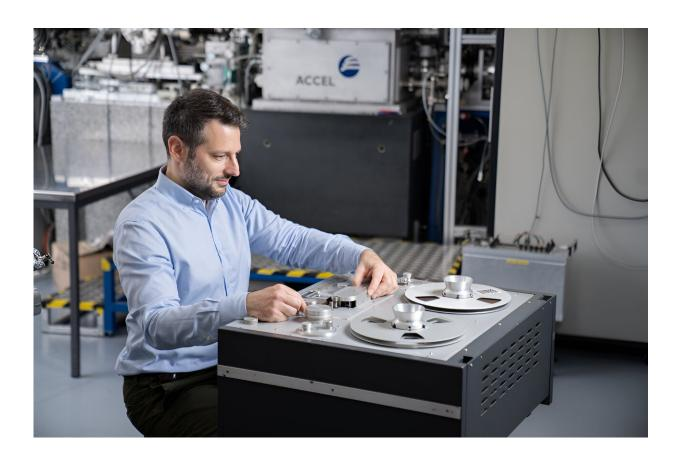
Sebastian Gliga winding a tape on a Studer A80: The tape machine is on loan from Idee und Klang in Basel, the studio of sound engineer and composer Daniel Dettwiler. The analog device, which was manufactured in Regensdorf in the 1970s, serves to produce reference recordings that can be directly compared with the results of the synchrotron measurements. Credit: Paul Scherrer Institute/Mahir Dzambegovic
