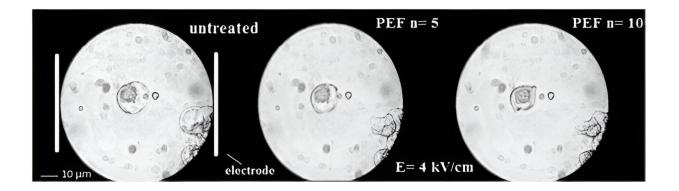
Protoplast serves as a model system for visualizing the impact of PEF-induced (4kV/cm) membrane rupture and cell shrinking. Credit: Afraz, M. T., et al.
