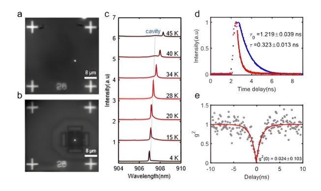
Figure 2. Single QD positioning and coupling to corner state. Credit: *Light: Science & Applications* (2024). DOI: 10.1038/s41377-024-01377-6
