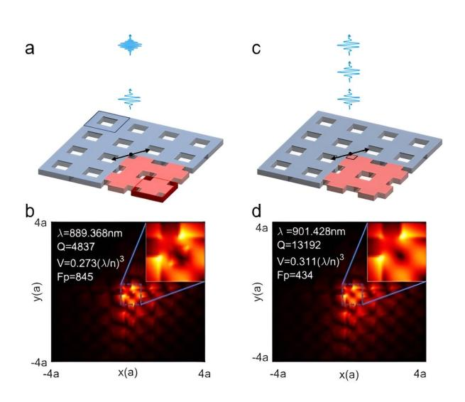
Figure 1. The theoretical scheme of the QD-in-topological cavity structure. Credit: *Light: Science & Applications* (2024). DOI: 10.1038/s41377-024-01377-6
