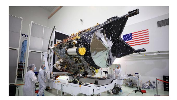
NASA's Psyche spacecraft is shown in a clean room at the Astrotech Space Operations facility near the agency's Kennedy Space Center in Florida on Dec. 8, 2022. DSOC's gold-capped flight laser transceiver can be seen, near center, attached to the spacecraft. Credit: NASA/Ben Smegelsky
