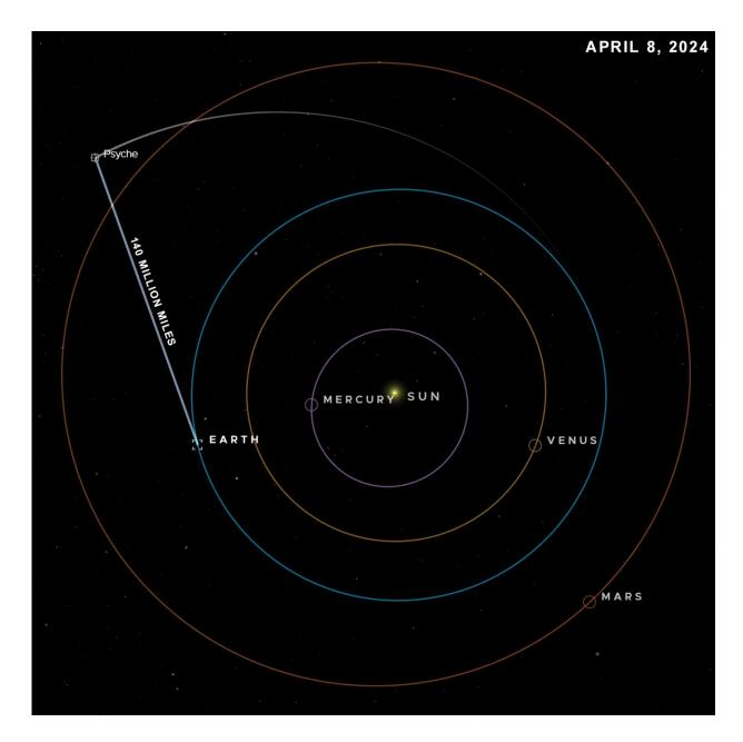
This visualization shows the Psyche spacecraft's position on April 8 when the DSOC flight laser transceiver transmitted data at a rate of 25 Mbps over 140 million miles to a downlink station on Earth. Credit: NASA/JPL-Caltech
