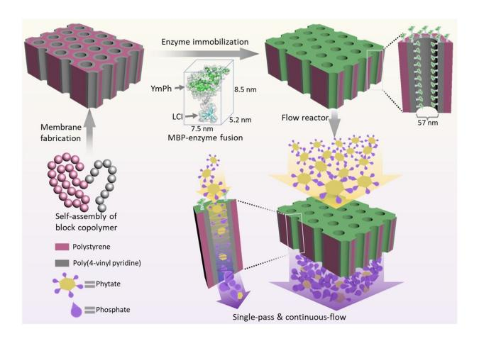
Schematic illustration of the general-applicable and scalable flow reactor design by combining well-designed isoporous BCP membranes as carriers with a fusion protein (phytase plus material binding peptide [MBP; namely LCI]) for oriented phytase (YmPh) immobilization. Credit: *Nature Communications* (2024). DOI: 10.1038/s41467-024-47007-y
