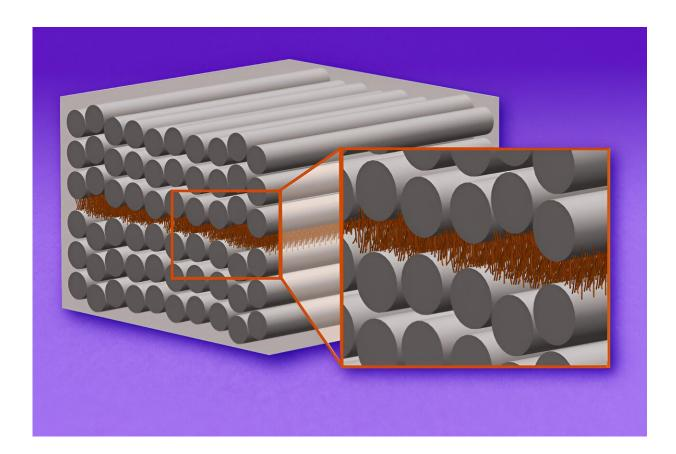
This schematic shows an engineered material with composite layers. Layers of carbon fibers (the long silver tubes) have microscopic forests of carbon nanotubes between them (the array of tiny brown objects). These tiny, densely packed fibers grip and hold the layers together, like ultrastrong Velcro, preventing the layers from peeling or shearing apart. Credit: Courtesy of the researchers, edited by MIT News
