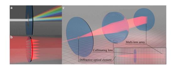
A multi-photon (7×7)-focus 3D laser printer based on a 3D-printed diffractive optical element and a 3D-printed multi-lens array. Credit: Light: Advanced Manufacturing (2024). DOI: 10.37188/lam.2024.003
