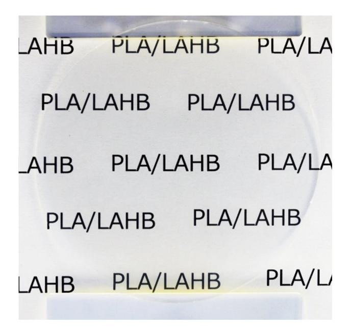
The material resulting from adding ultra-high molecular weight LAHB to lactic is a highly transparent plastic: The circular disk is almost invisible in front of a sheet of paper that has "PLA/LAHB" printed on it. Credit: Koh Sangho
