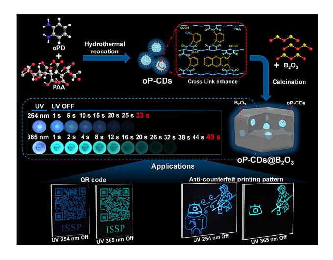
Schematic diagram of the preparation of multi-color long-lived roomtemperature phosphorescent composite materials based on carbon dots and their potential applications in anti-counterfeiting. Credit: ZHANG Qipeng
