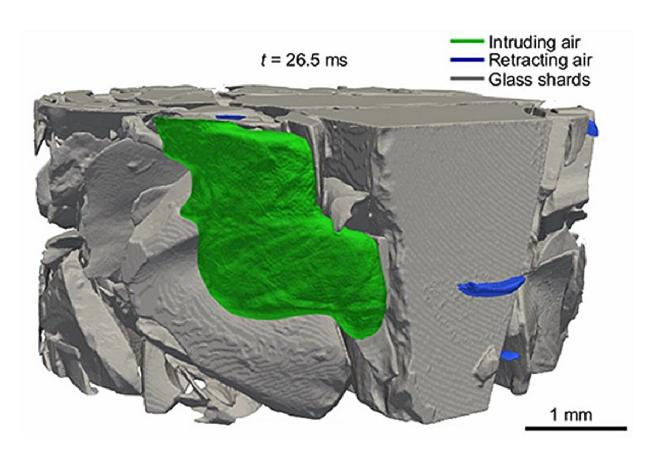
Towards the end of a Haines jump, a pore has been filled with encroaching air. This air is shown in green, while the surrounding material is grey. Credit: NTNU
