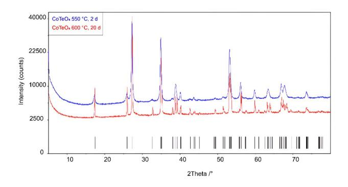
X-ray powder diffraction patterns of single-phase CoTeO<sub>4</sub> tempered for 2 days at 550 °C and for 20 days at 600 °C. Tick marks represent the position of Bragg reflections. Credit: *Materials Advances* (2024). DOI: 10.1039/D3MA01106B
